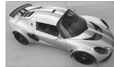
The Lotus Sport Exige Cup, priced at \$79,995, is a track car and not street legal. It has a supercharger that bumps power up to 243 bhp and maximum torque to 178 lb.ft. It features a limited slip differential, fully adjustable suspension, a fire suppression system and a full roll cage. Despite the addition of the supercharger and roll cage, weight is kept under 2000 lbs by removing things like the headlights, air conditioning and the battery cover.
