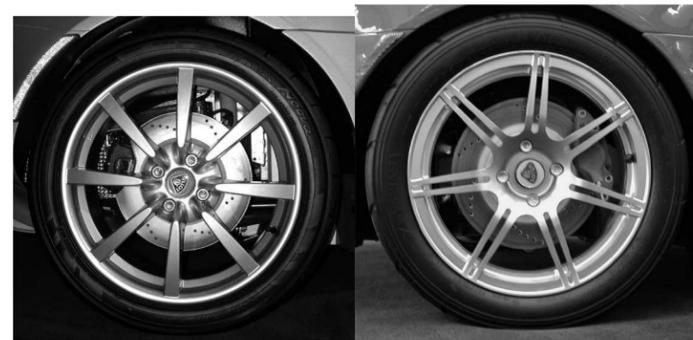
The hubs have been changed to use the more common 4x100mm bolt pattern from the obscure 4x96.25mm pattern used on the original Elise.
