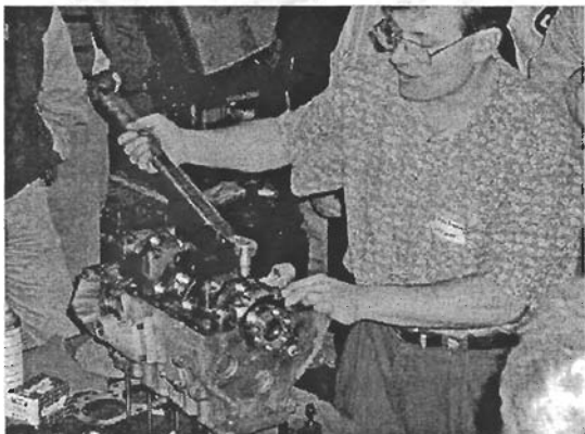
Torquing the steel main bearing caps.
