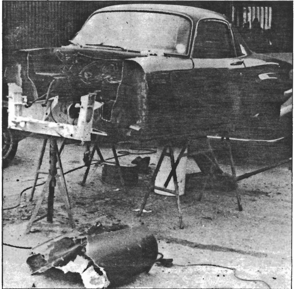
Showing the damaged areas cut away leaving a clean "square" edge.
